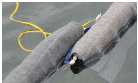
Shore Guard aka "Dumbo Surfer" connected units - 10" overlap - stainless steel clips
